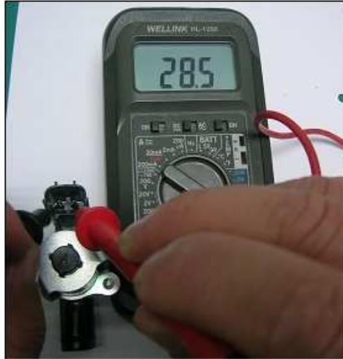
Figure 25 Measuring the resistance value of AISV
