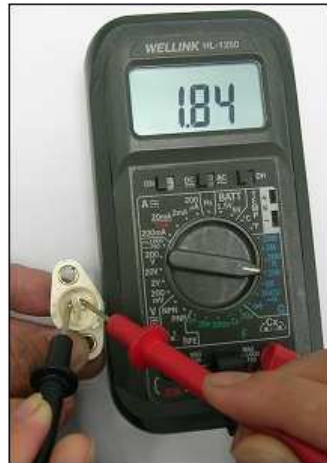
Figure 24. Measuring the resistance value of AT sensor
