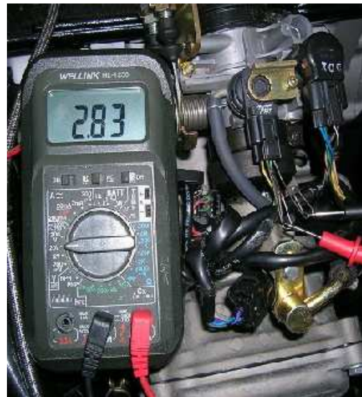
Fig.4 PM Sensor voltage signal output at sea level
