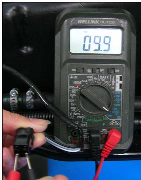
Figure 13 O 2 Sensor electrical resistance measurement
