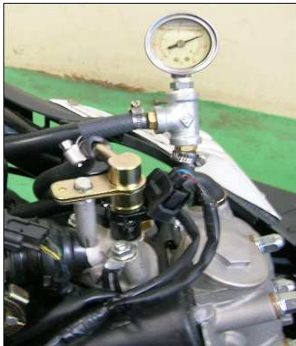
Figure 18. Fuel pressure measurement
