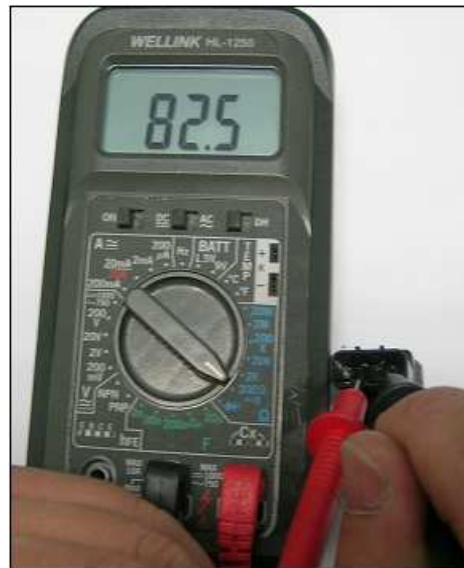
Measurement of Resistance in B phase
