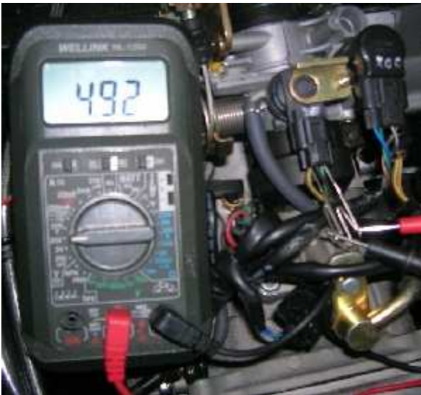
Fig.3 PM Sensor working Voltage measurement
