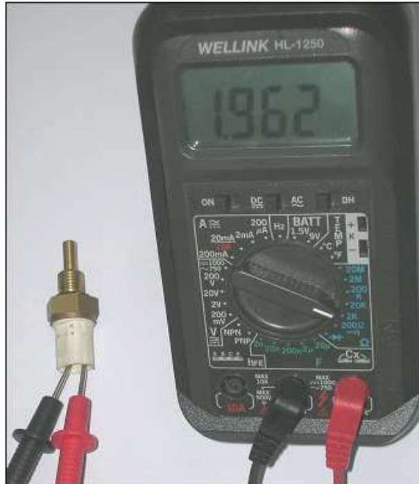
Fig. 8 Measuring the electrical resistance of TW
