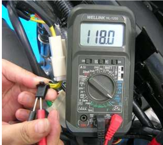
Figure 23. Measuring the resistance value of pulse sensor
