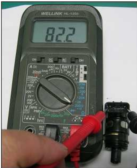
Measurement of Resistance in A phase
