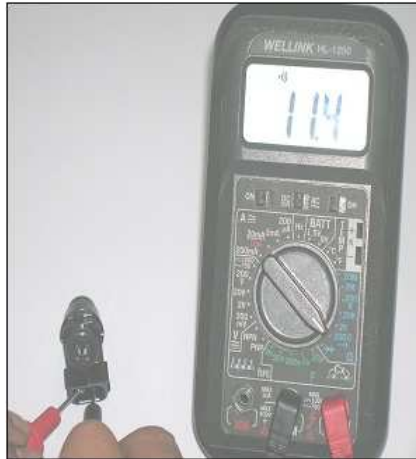
Figure 20. Measuring fuel injector electrical
