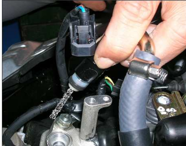
Figure 22. Bad nebulization- abnormal injector
