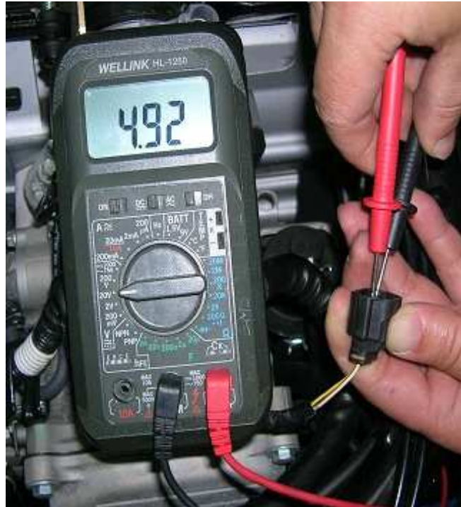
Fig. 5 TPS working voltage measurement from ECU side
