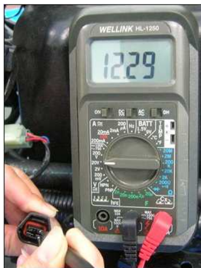
Figure 15a Measurement of Fuel Pump Working Voltage Liquid level
