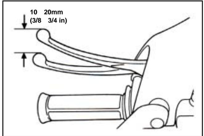
Adjust the free play by turning the front brake adjustment nut if necessary.
