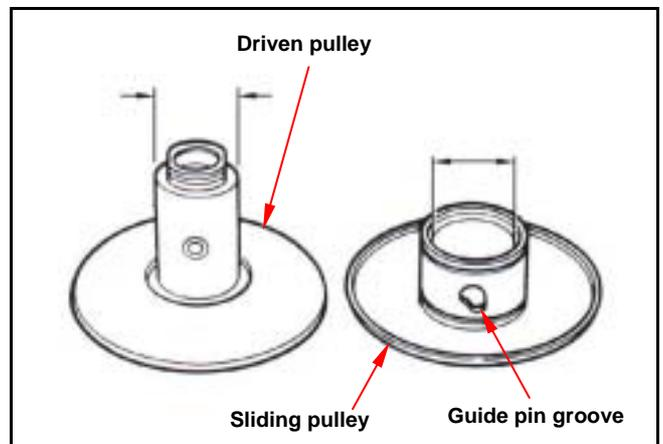
**Driven Pulley Bearing Inspection**
