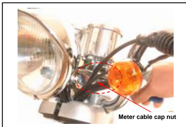
Remove 2 cap nuts from meter ASS'Y and then remove meter ASS'Y.
