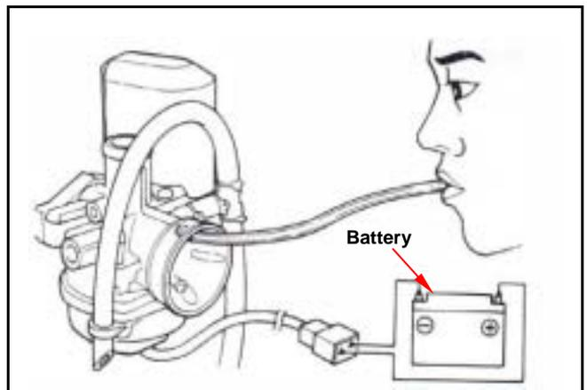
Check resistor to make sure that the auto by-starter is in normal. Engine is running.
