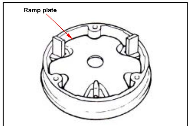
Apply with grease 4~5g to inside of movable drive face, and install drive face boss.
