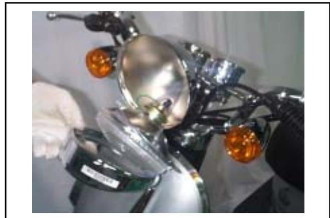
Remove bulb seat and replace the bulb.
