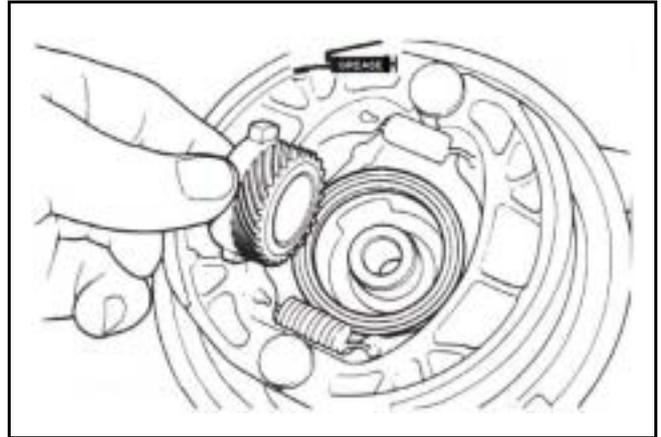
Align the flange part on the speedometer gear with the slot of wheel hub.
