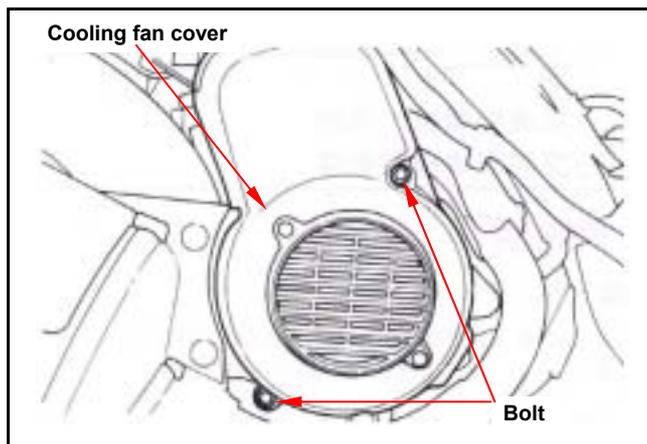
Remove four bolts, and then take out the cooling fan.
