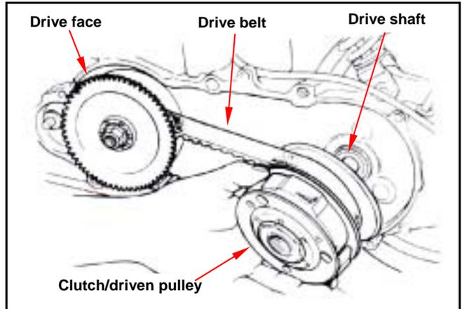
Install the clutch with universal holder, and then tighten nut to specified torque value.
