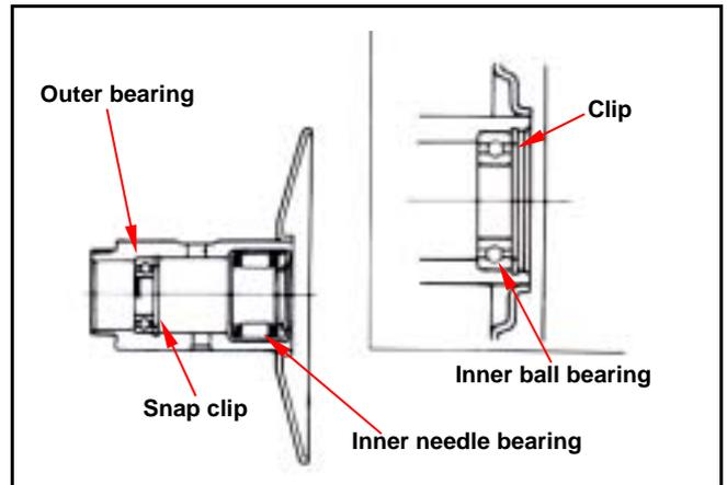
Place new bearing onto proper position and its seal end should be forwarded to outside. Apply with specified grease.
