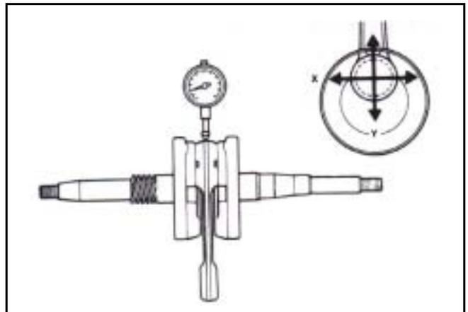
Place the crankshaft on a V-block, measure run-out points A and B of the crankshaft with dial gauge.
