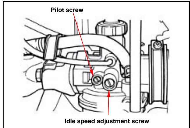
Adjust the idling after warm up engine for 10 minutes.
