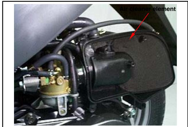
Soap the element into cleaning engine oil and then squeeze it out. Install the element onto the element seat and then install the air cleaner cover.
