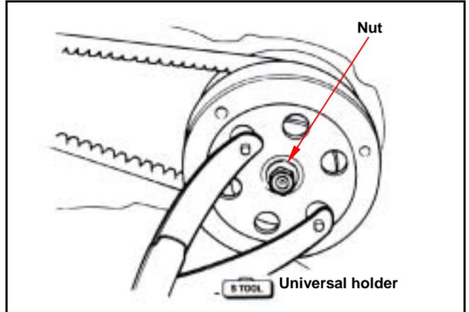
Push the drive belt into belt groove as diagram shown so that the belt can be loosened, and then remove the driven pulley.
