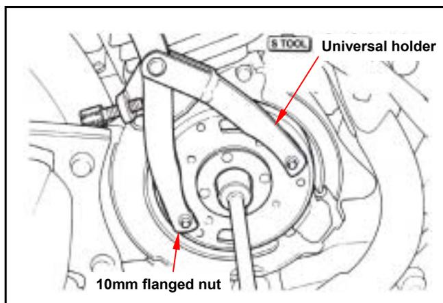
Remove the flywheel with rotor puller.
