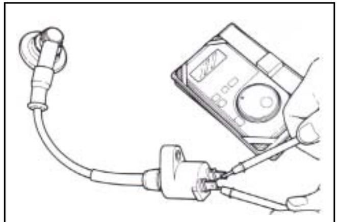
Remove the high voltage coil cap, and measure its negative (-) terminal for the secondary coil resistance.
