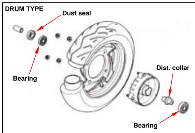
Remove dust seal, bearing and side collar.
