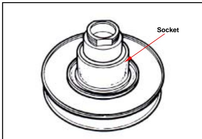
Install driven pulley, spring and clutch into clutch spring compressor, and press down the assembly by turning manual lever until mounting nut that can be installed.
