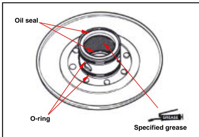
Install sliding pulley onto driven pulley.
