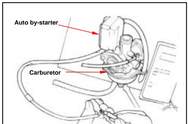
Remove carburetor, and allow it to cool off for 30 minutes.
