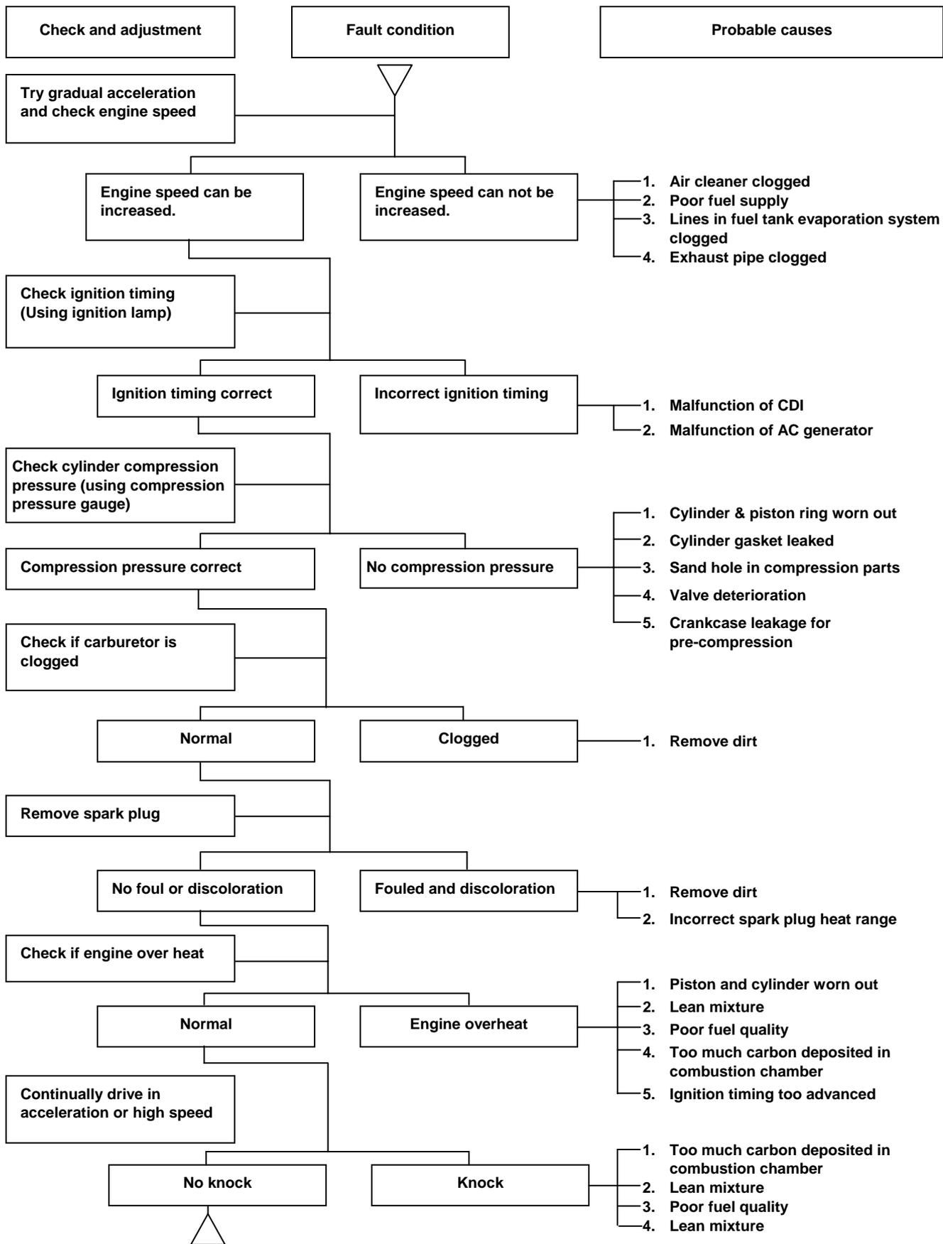
**C. Engine runs sluggish (especially in low speed and idling)**
