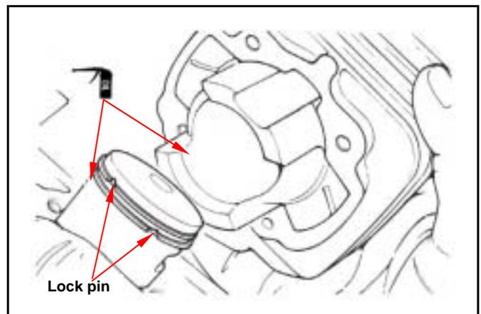
Lubricate cylinder and piston with two-stroke engine oil. Hold the piston and then install it into cylinder.
