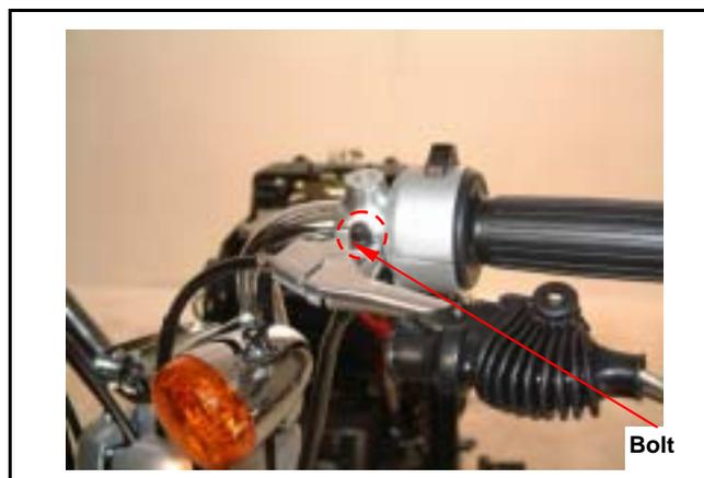
Remove front and rear brake lever bracket mounting bolt.
