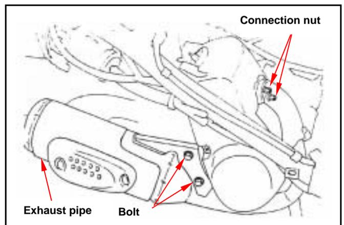
Remove engine mounting nut and bolt.
