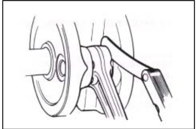
Measure the radial clearance of connecting rod big end at X-Y directions as diagram show.
