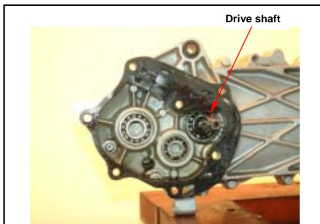
Remove drive shaft oil seal and bearing from left crankcase.
