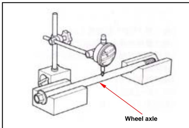
Place the wheel on to a rotation seat, and turn the wheel to check its bearing free play. If the bearing is noisy or its free play is too much, replace it.
