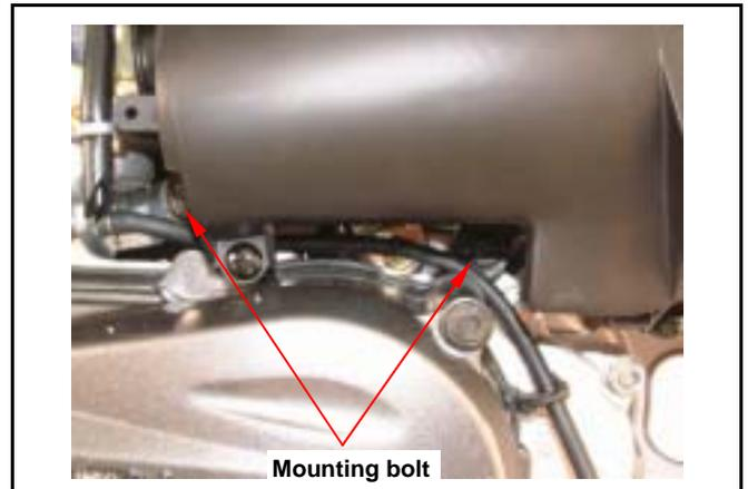
Support the engine and then remove shock absorber lower mounting bolt.
