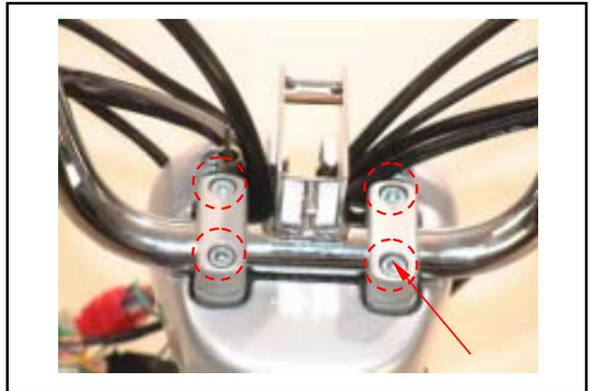
Remove handle and front brake lever bracket.
