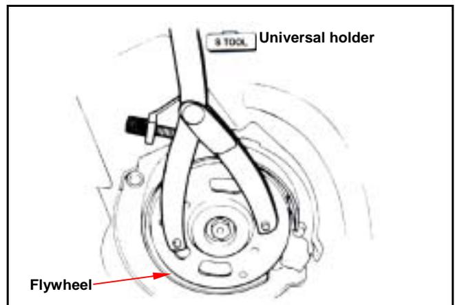
Tighten nut to specified torque.
