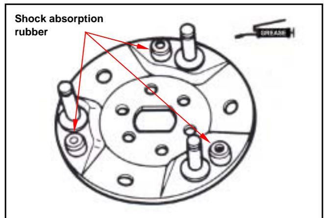
Install new clutch weight onto lock pin and then push to specific location. Apply with grease onto lock pins. But, the clutch weight should not be greased. If so, replace it.
