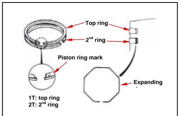
Push the rings into ring groove and then check rings' mating condition.
