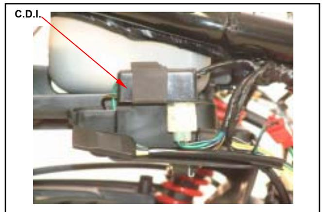
**CDI Electrical System Circuit Inspection**
